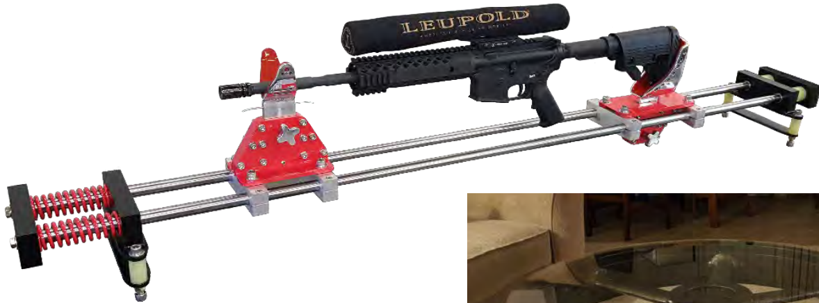
Stationary Recoiling Device for the Testing of Long-barreled Firearms
