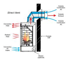
**DIRECT VENT TECHNOLOGY** allows you to add a fireplace to rooms with no existing chimney. Simply vent your fireplace through an outside wall and finish it with the patented **Regency AstroCap Flex Venting System**.
