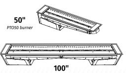
Two PTO50 burners connected end to end
