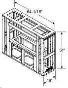
Custom application using the Regency Plateau™ PTO30 burner and see-through framing kit with Stainless Steel Panels.
