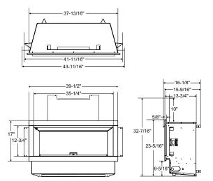
NOTE: Gas Connection/Electrical connections if using optional Hardwire Kit are located on left hand side of appliance.
